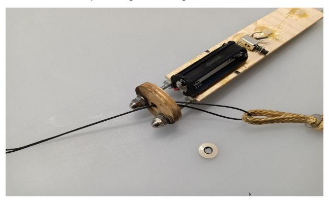
Step 4: Pull the pull through cord until the soft anchor has fed through the bulkhead and the SS washer is flush against the backside of the bulkhead.
