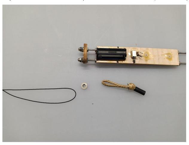
Step 3: Route the pull through cord through the loop in the soft anchor and then feed both ends of the pull through cord through the anchor hole in the bulkhead.
