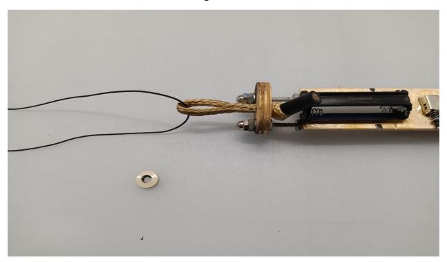
Step 5: Leave the pull through cord routed through the soft anchor and route the pull through cord's ends through the rubber washer, and pull the cord while pushing the rubber grommet flush to the face of the bulkhead.
