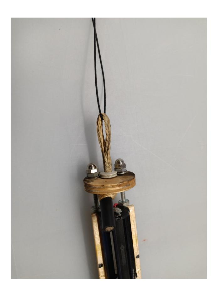
Step 6: Remove the pull through cord and the installation is complete. Remember to inspect before each flight.
